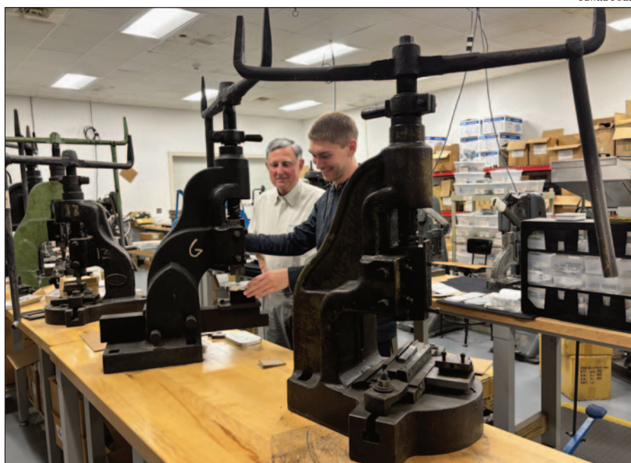
Alan Gnann (left) assisting lead technician Chris Beebe with production of a Wheatley fly box on one of the original nineteenth-century Wheatley factory fly presses.
