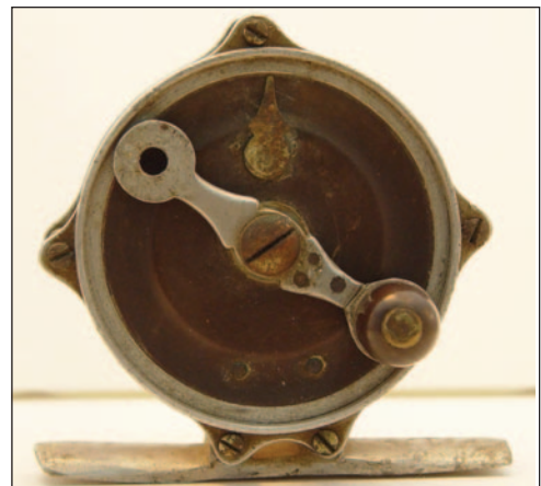
Frederick Malleson designed his patent multiplying reel in 1883, with a four-gear train tucked under a raised housing on the tail plate. It also featured a little arrow-shaped click switch. Photo by Nathan George.
