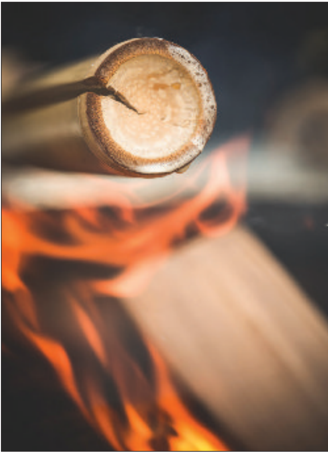
Above: Water boils out of the fibers of the culm.
