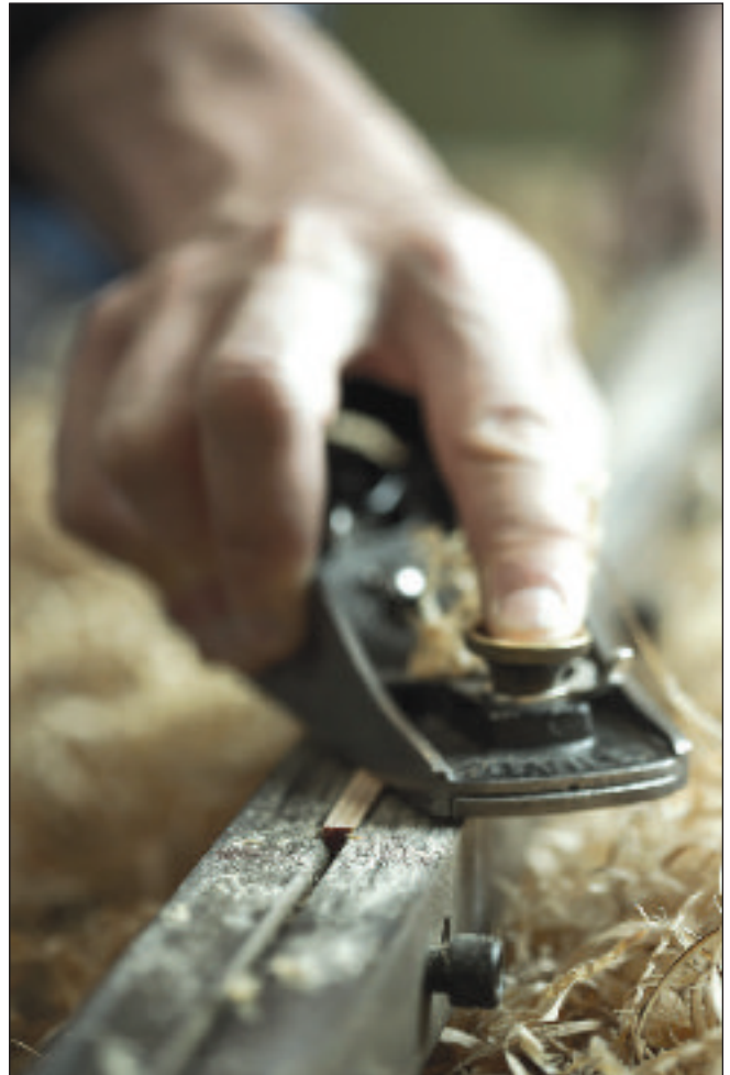
Right: Shaving the bamboo into tapered strips.
