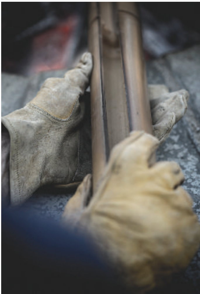
Leather gloves are needed to handle the heated bamboo.
