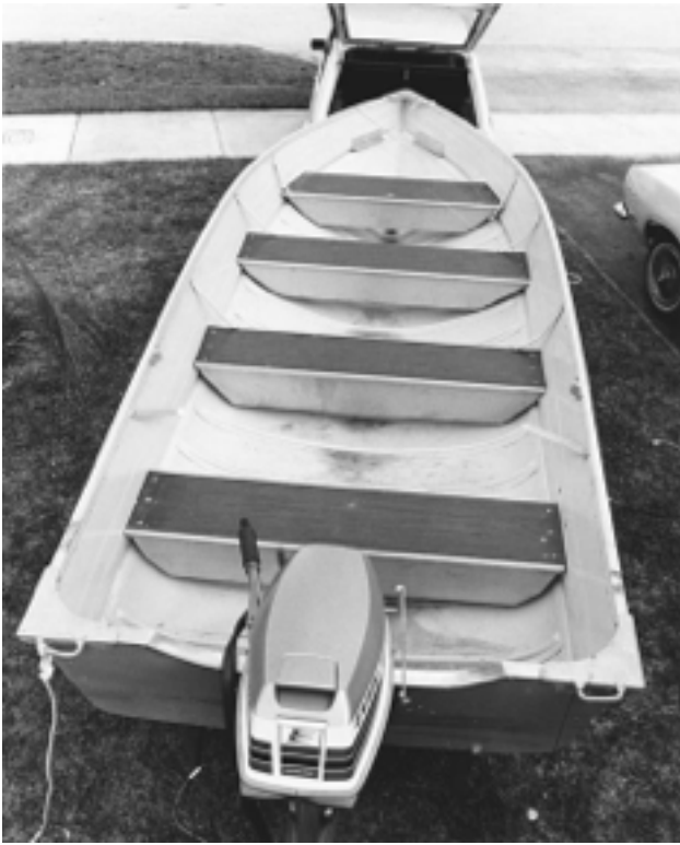
The Alum1: A 16-foot semi-vee aluminum utility boat before it is converted into a flats boat.
