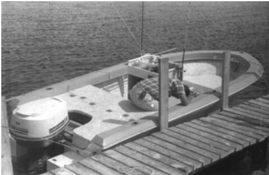
One of many bare hulls converted for flats fishing by adding a rear deck and center console. This Capri 16 came from the factory with the flat gunwales and recessed foredeck.
