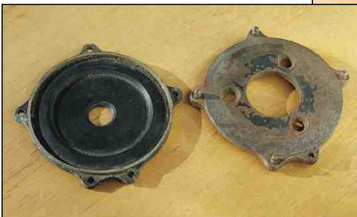
Figure 24. An iron lathe fixture for locating and holding a plate assembly while turning and facing to final contour. Boring for the center bearing and polishing could also have been performed during this setup. From the collection of Hoagy B. Carmichael, with permission.
