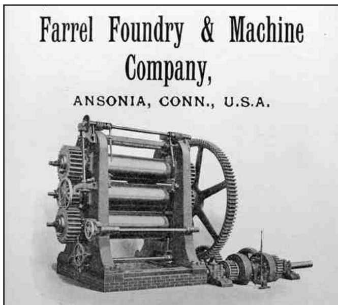
Figure 29. Three-roll calenders rolled rubber compounds into sheets before being cut up for compression molding. Source: Franz Clouth, Rubber, Gutta-Percha and Balata (New York: D. Van Nostrand Company, 1903), 248.
