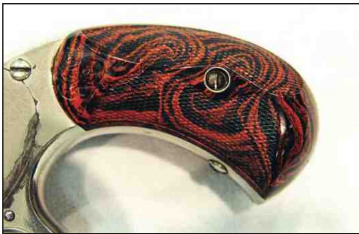
Figure 46. Smith & Wesson mottled red and black hard-rubber grips were impressive and handsome. Although not commonly encountered, these grips were often fitted to Smith & Wesson's nickel-plated arms.
