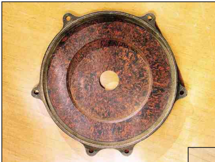
Figure 22. A Leonard salmon reel plate. Note the fine shrinkage fissure at about 8 o'clock. The shrinkage of mud as it solidified would have been accentuated with larger diameters. From the collection of Hoagy B. Carmichael, with permission.
