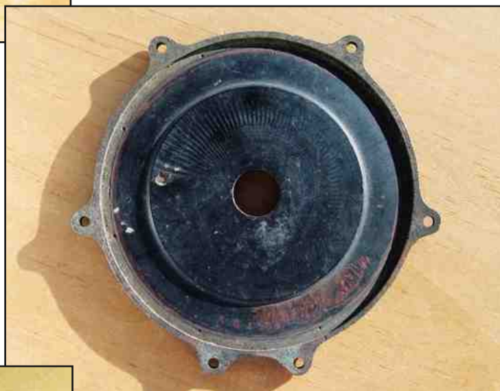
Figure 23. An early reel with two layers of mud; the orange and black mixture was used against the face of the reel, the supporting brown composition was unseen inside the reel. The second layer may have been a formula to add impact resistance or reduce shrinkage. From the collection of Hoagy B. Carmichael, with permission.
