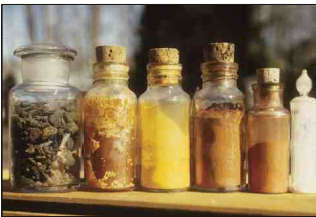
Figure 7. “Mud” was mixture of hot-melt resins similar to rosin or shellac that could be molded. Hardness was adjusted by the choice of resins and diluents; pigments offered a broad range of colors.
