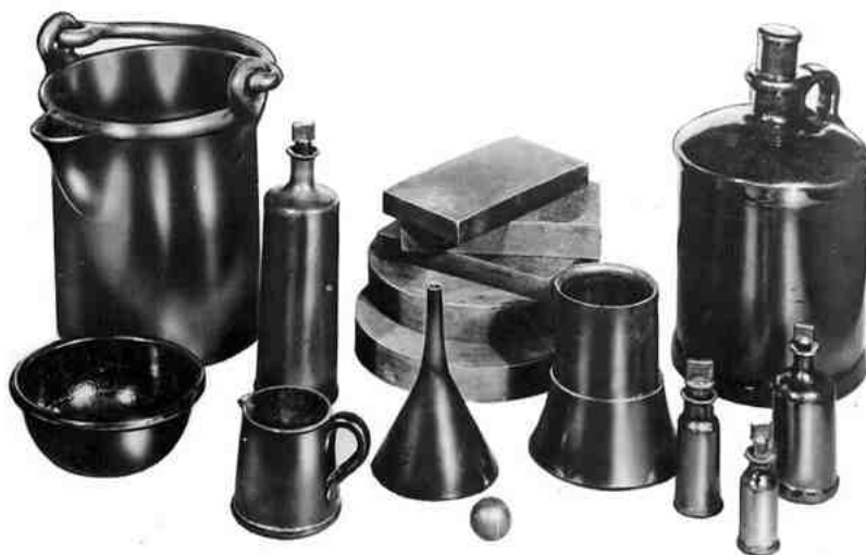
Figure 3. Typical products molded from gutta-percha during the 1850s and 1860s. Note the natural satin finish. Gutta-percha offered wonderful resistance to biodegradation. Source: Jim Jones Collection: Atlantic-Cable.com website.
