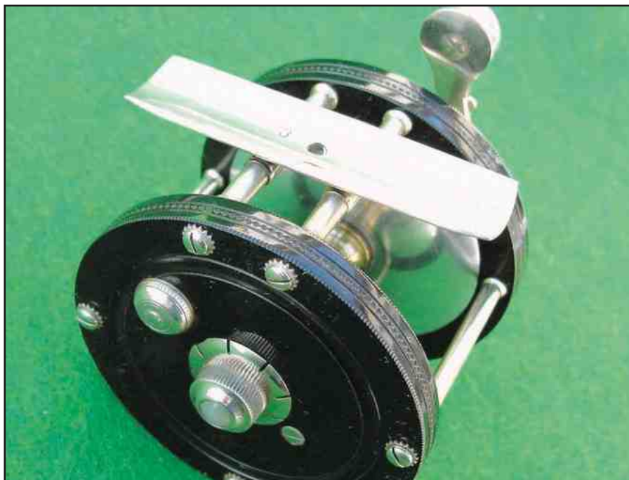
Figure 44. Julius Vom Hofe multiplier with embellishments applied after molding. Hard rubber was easy to engrave, roll imprint, and stamp with makers' names and trade logos.
