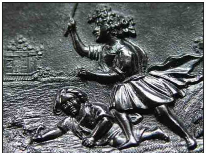
Figure 8. The surface detail of products molded from mud was excellent. This is the surface of a Littlefield, Parsons & Company picture frame.
