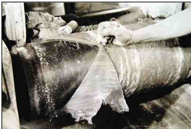
Figure 28. A two-roll mill used to mix sulfur and compounding ingredients with raw rubber in the solid. After vulcanizing, the hardness of the cured rubber varies with the sulfur concentration.
