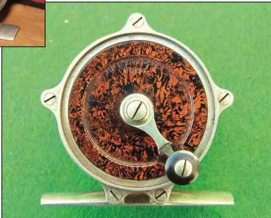
Figure 15. Impact resistance was adequate to allow stamping of H. L. LEONARD, MAKER.
