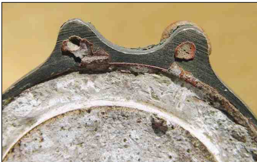
Figure 21. A white powder, probably talc, is found on the interior of several discarded plates; this would seem to be a mold release, likely added to ease prying the mold open. From the collection of Hoagy B. Carmichael, with permission.
