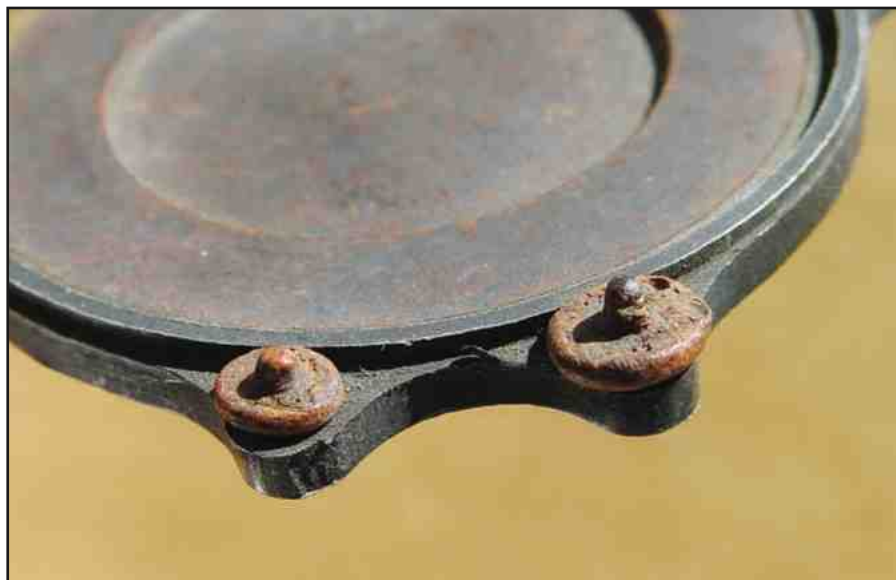
Figure 19. In compression molding, the excess hot mud oozes from the mold into the pillar holes predrilled in the frame. The shape of the buttons reveal the mold construction and position of unused locating pins.
