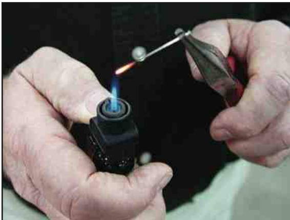
Figure 26. A simple test for mud involves gently probing with a hot needle to see if it melts.
