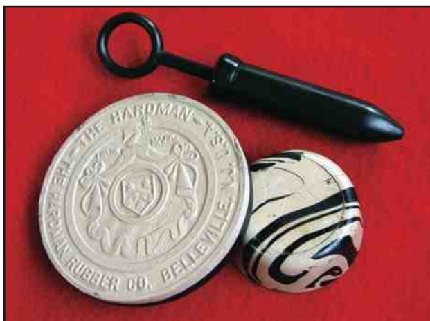
Figure 45. Not all hard rubber was black, although carbon black was a superb reinforcing filler. Lighter colors could be provided.
