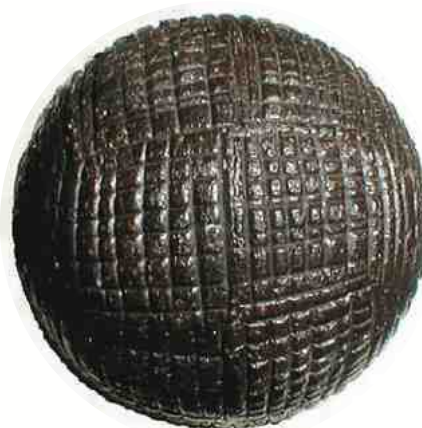
Figure 4. A gutta-percha golf ball. These "gutties" had remarkable impact and slash resistance.
