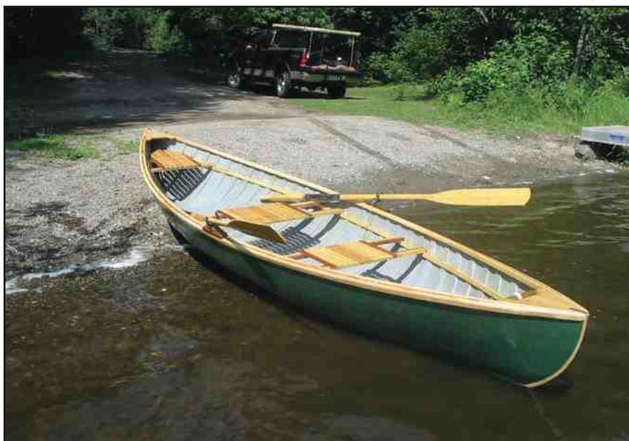
The basket-case peapod after restoration by Fred Kircheis. Note the typical close seat placement for rower and angler.
