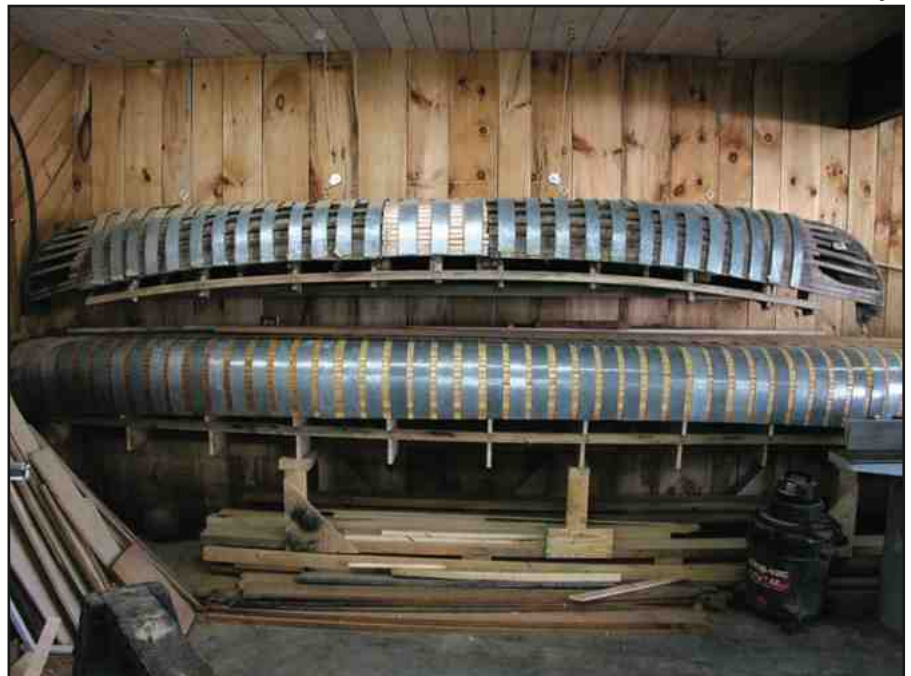
Karl Andersen boat form suspended over a Grand Laker canoe form in Steve Forrest’s barn. Note the added middle section restoring original boat dimensions.
