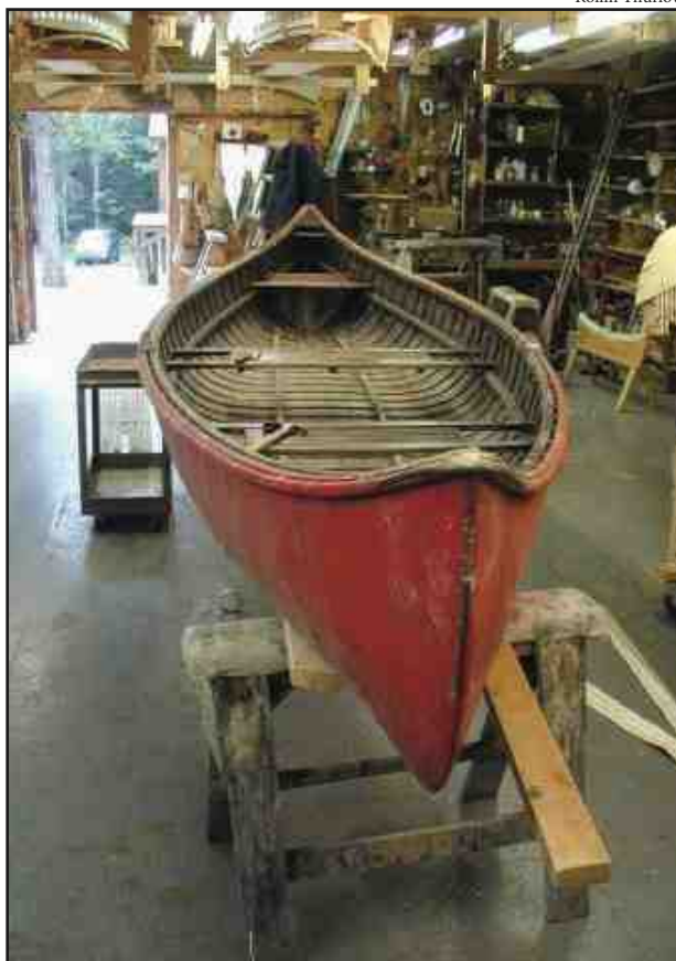
Early peapod built by E. H. Gerrish that retains the flat bottom and upturned ends typical of classic canoe form.
