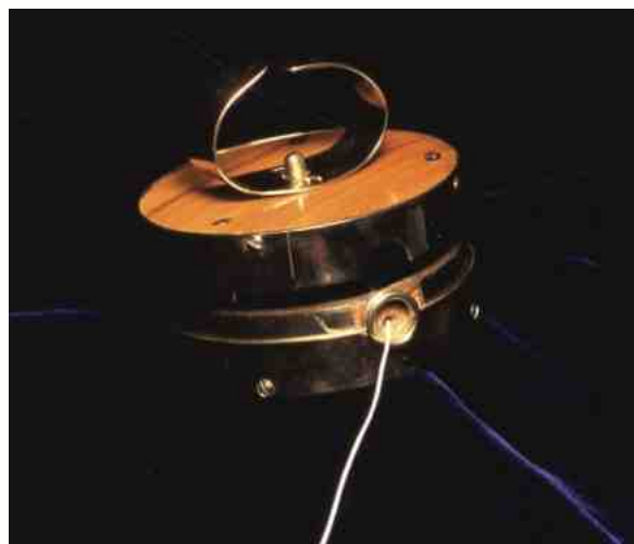
Figure 9. The brass flange sprung into the inside of the cavity of the housing.
