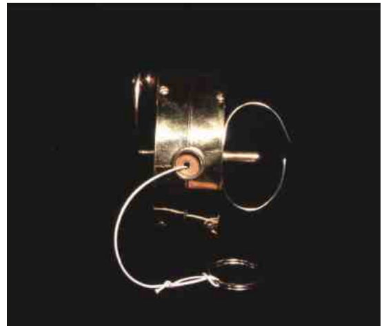
Figure 6 (top right). The crank side of the reel showing two of the six screws that hold the halves of the housing together (three screws per half).
