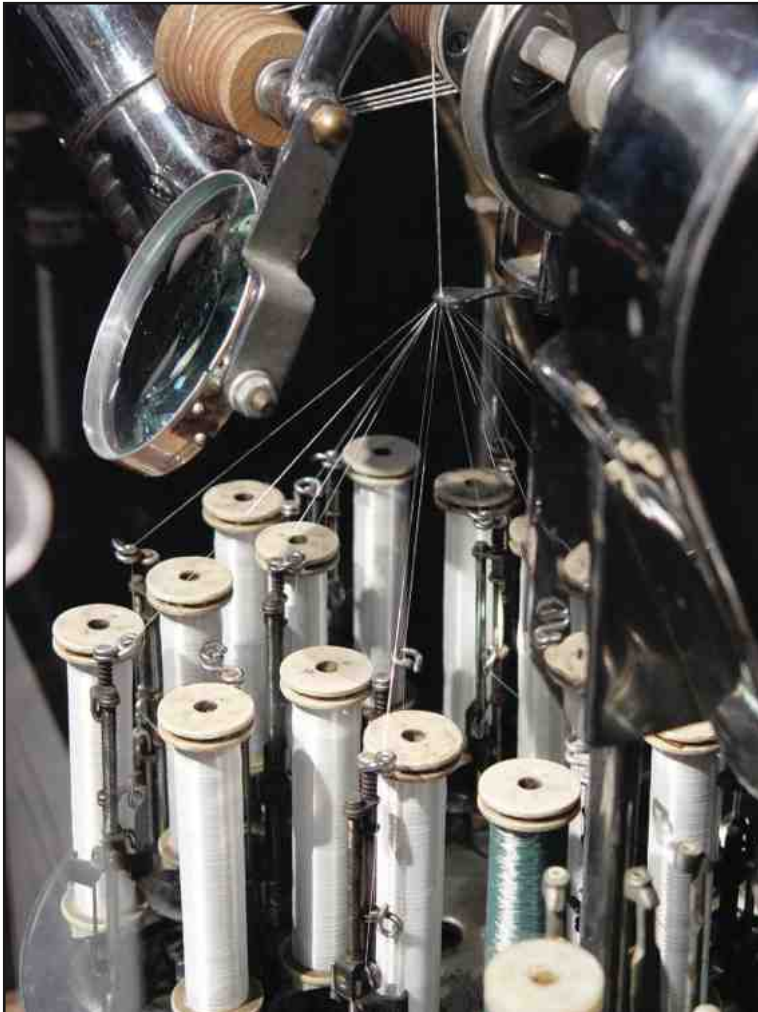
Above: Sixteen spools of filament weave in and out, creating the finished braid. The track layout determines the braid pattern; spools of colored filament can introduce coded stripes or product markers.
