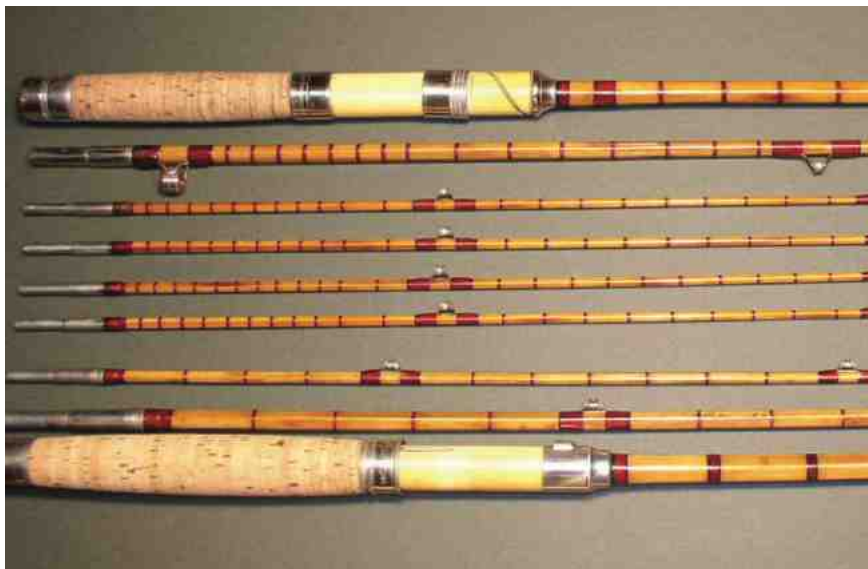
Comparison of wraps and reel seats on Landman-made VL&A (upper) and Kosmic; doubled intermediates of VL&A are repeated at each ferrule and tip.
