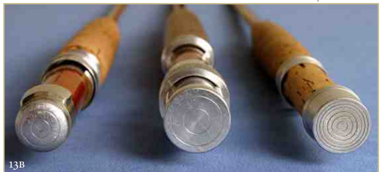
Inset: Left: Dual rows of straight, vertical knurling on a Halstead trout rod marked with his die stamp. Right: Unmarked Halstead trout rod with the custom frosted textured finish and dual rows of fine, ropelike diagonal knurling.
