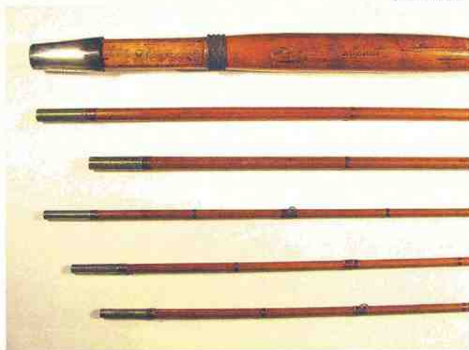
Attractive one-piece bird's-eye maple hand grasp and reel seat with a finely knurled sliding band and unusual butt cap. Simple, straight rolled and soldered male ferrules with exposed wood bottom.
